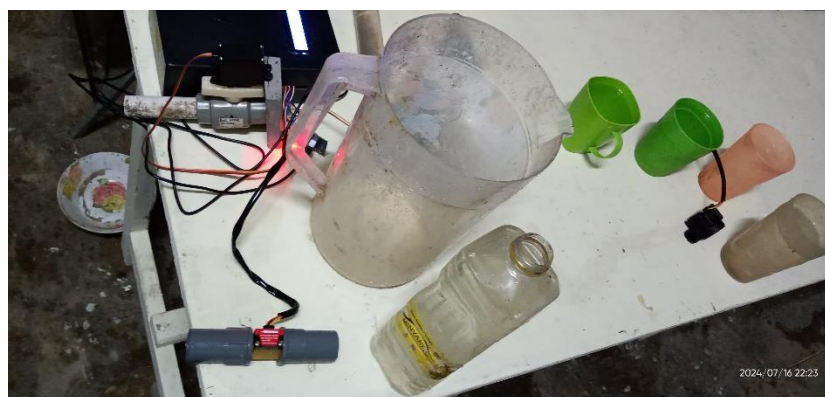
Gambar 4. 8 Kalibrasi Sensor Waterflow
