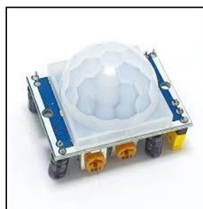
Gambar 2. 2 Passive Infrared Receiver (PIR)
